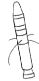
The first American satellite, Explorer 1, went into a flat spin because its flexible antennas triggered nutational growth.
