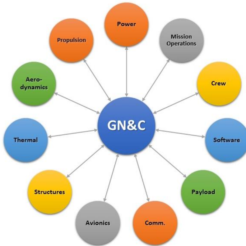
Figure 1.3-1. GN&C Subsystem Influence Diagram
