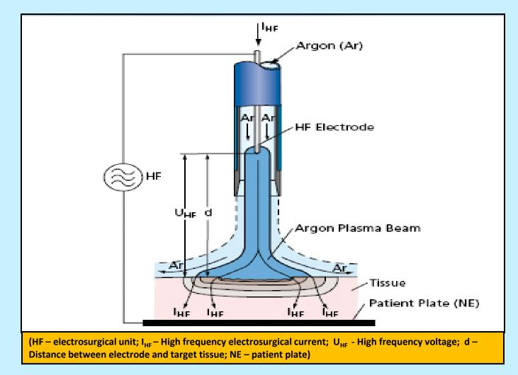
APC is a monopolar application in which HF electrical energy is transferred to the target tissue using ionized (conductive) argon gas (plasma), without the electrode coming in contact with the target tissue
