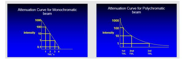
Note that for monochromatic photons, all TVLs are equally thick; for polychromatic photons, layer 3 is thicker than layer 2, which is thicker than layer 1,
