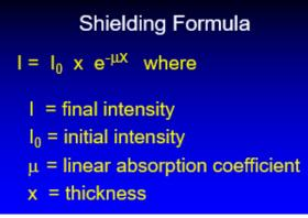
If we solve for  $e^{-\mu x}$ , we see that it is equal to the fraction penetrating.
