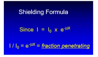
Using a logical approach to understanding attenuation, as displayed below, we see that the fraction penetrating is also equal to  $0.5^{n}$
