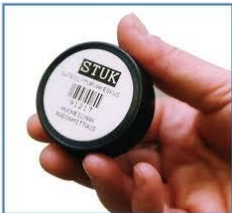
Figure XIII.11. a) Indoor radon monitor having a polycarbonate film detector b) Tracks due alpha particles from radon in polycarbonate film, magnification 40, the photographed area is about 1.3 by 1.0 mm ( http://pages.csam.montclair.edu/~kowalski/cf/327squeeze.html ).
