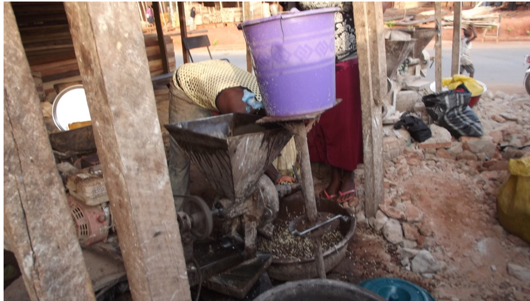
Figure 13: Domestic grinding machine used as dehuller Source: Enibe D. O. (2013)
