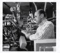
Performing in-situ X-ray emission measurements.
