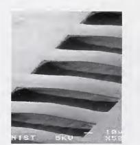
Fixed-fixed beam test structure array for measurement of mechanical strain and interconnects in multilayer structures.
