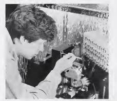
Loading a sample into the Scanning Capacitance Microscope.
