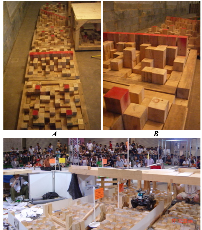
Figure 5: A, B) The Stepfield Dash is used for robot qualification for the RoboCupRescue Robot League competitions. C) The 2005 Championship arenas in Osaka, Japan.
