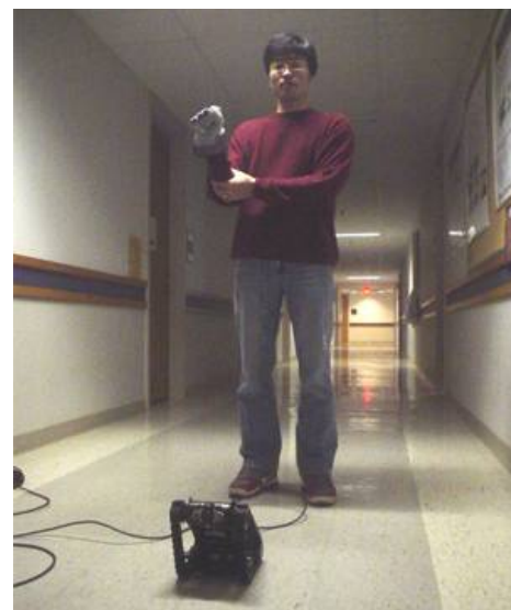
Figure 1: Using the Gestural Joystick to operate a commercial Inuktun robot.
