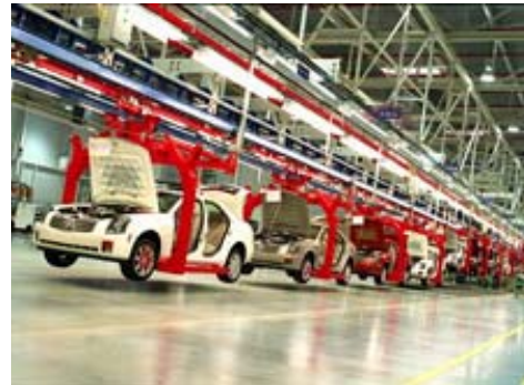
Figure 1 Automotive General Assembly Conveyors Transport Vehicle Bodies for Assembly Operations
