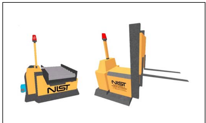
Figure 2: Forklift and unit loader AGVs created for USARSim.
