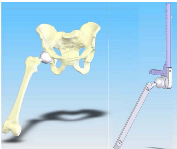
Figure 1. The image on the left is a depiction of a patient pelvis along with a femur bone and an artificial ball joint. Comparing this to the NIST phantom and femur bar on the right side of the figure, it is easy to recognize the motivation for the construction of the measurement artifact.
