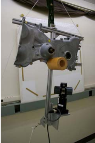
Figure 2. SmartTRACK sensor below engine part
