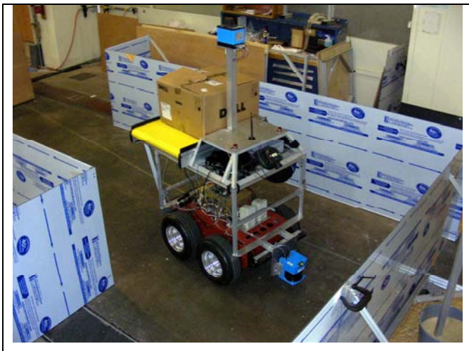
Figure 9: The winning code from Hood College was placed without change on NIST's surrogate AGV. The vehicle was able to successfully navigate and dock with a loading area.
