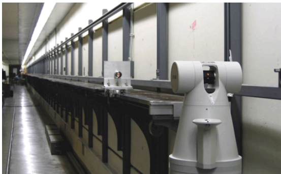
Figure 2. The NIST 60 m laser rail facility viewed from the tracker under test end; note the movable carriage with retroreflector.
