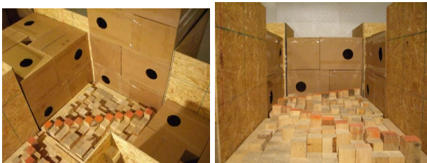
Figure 8: The Manipulator Dexterity: Perception test method is shown with half-cubic stepfield terrain for added complexity.
