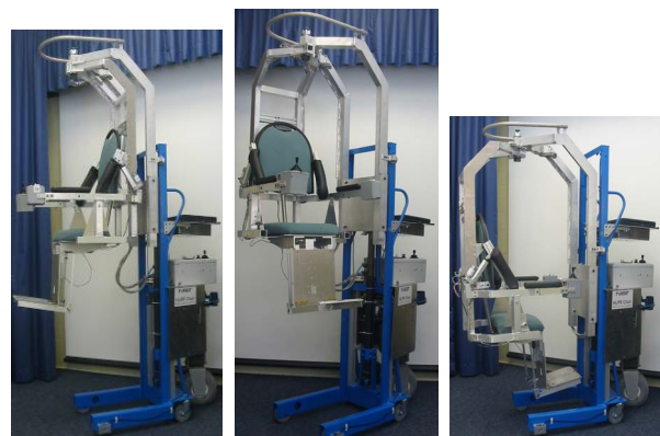
Figure 4: Load/Seat Orientations of the HLPR Chair with respect to the frame including: (left) forward, (middle) side, and (right) rear orientations.
