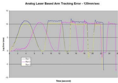
Figure 25 The Position Lag Error for the Analog Sensor Based Arm Tracking: 120mm/sec Case
