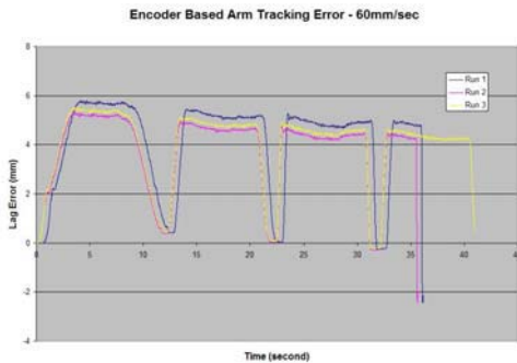
Figure 9 The Position Lag Error for the Encoder Based Arm Tracking: 60mm/sec Case
