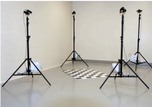
Figure 1: Photo of a calibrated camera network with four cameras. The checkerboard pattern in the center is a calibration target.
