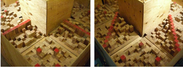
Figure 6: A) The Endurance test method has one lobe of the figure-8 with perpendicular hill pallets separated by generally flat pallets. B) The other lobe has diagonal hill pallets separated by generally flat pallets. The center path of the figure-8 uses flat pallets (not shown).
