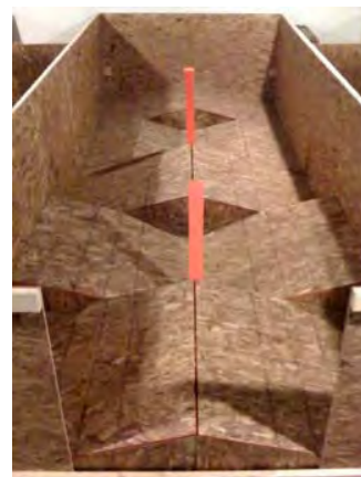
Figure 3: Crossing Ramps Terrain Test Method
