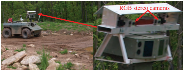
Figure 1. JPL water detection software has been integrated onboard XUVs and evaluated at Ft. Indiantown Gap, PA. A forward-looking stereo pair of color cameras provides water cues from color, texture, and object reflections.
