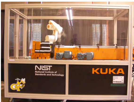
Figure 5: 1/3 scale palletizing cell used during the ICRA Competition
