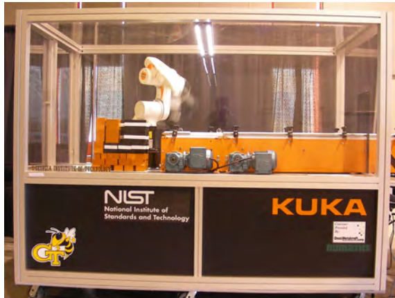
Figure 4: 1/3 scale palletizing cell used during the ICRA Competition
