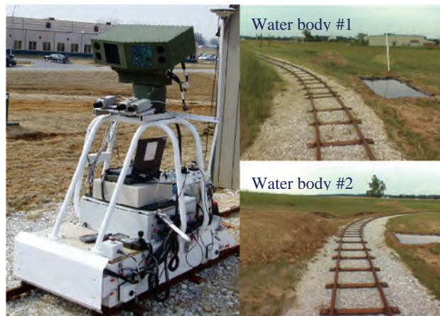
Figure 9. A JPL passive perception system was mounted to a GDRS instrumented train. Color stereo imagery was collected on a surveyed obstacle course containing two rectangular man-made water bodies at speeds of 1, 3, and 5 m/s.
