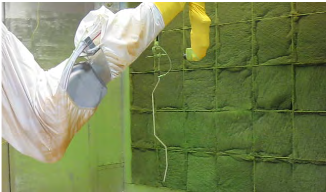
Figure 3: Robotic Painting of Scanned Tubes
