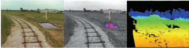
Figure 10. A frame showing the first man-made water body on the test course described in Figure 9 during a 1m/s run (left), water detection results overlaid on a grayscale intensity image (middle), and a wide-baseline stereo range image (right). In the color coded water detection overlay, blue, magenta, and red correspond to one, two, and three cues for water, respectively. In the stereo range image, black corresponds to no range data.
