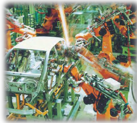
Figure 1 Traditional Human Robot Exclusion in Automotive Robotic Manufacturing Workcells
