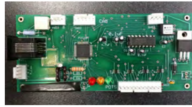
Figure 3: The custom circuit board containing a PIC microcontroller, a single-axis gyroscope, and four digital potentiometers.
