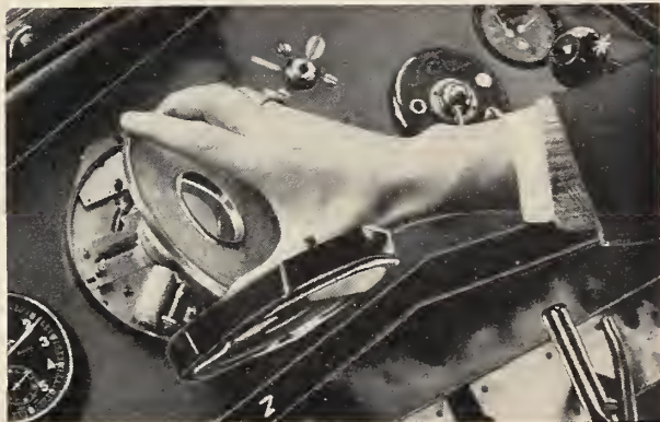
FIGURE 1. Wet-paint disk recorder with self-erasing device (Hasler Co.)
