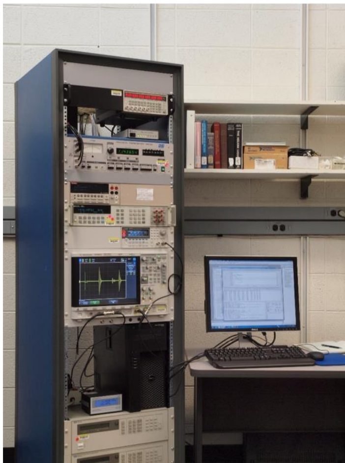
Figure A.1-5. Instrument rack for the pulse-echo speed of sound instrument
