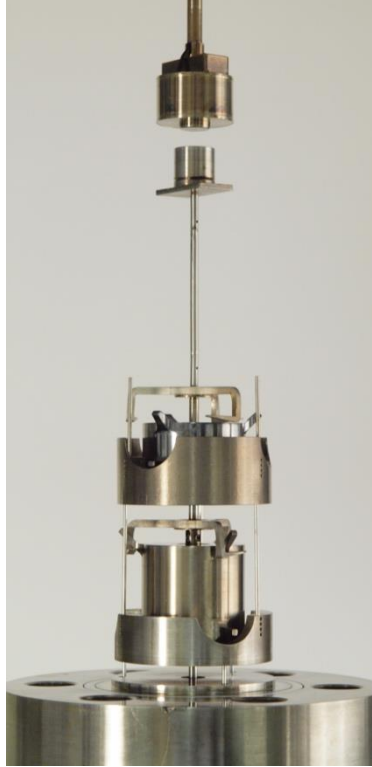
Figure A.1-3. Sinkers in the two-sinker densimeter (shown removed from the measuring cell)
