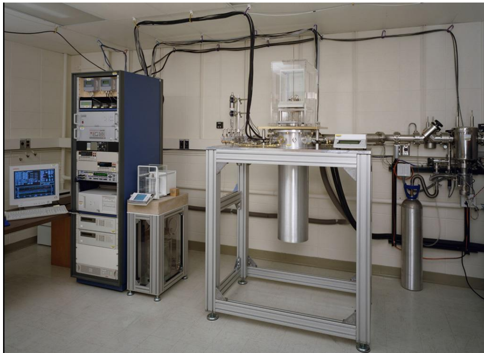
Figure A.1-2. Two-sinker densimeter
