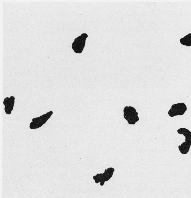
FIGURE 5. Irregularly shaped particles of +40-micron fraction of electrolytic copper, Cu B, powder. Magnification \times 100 .
