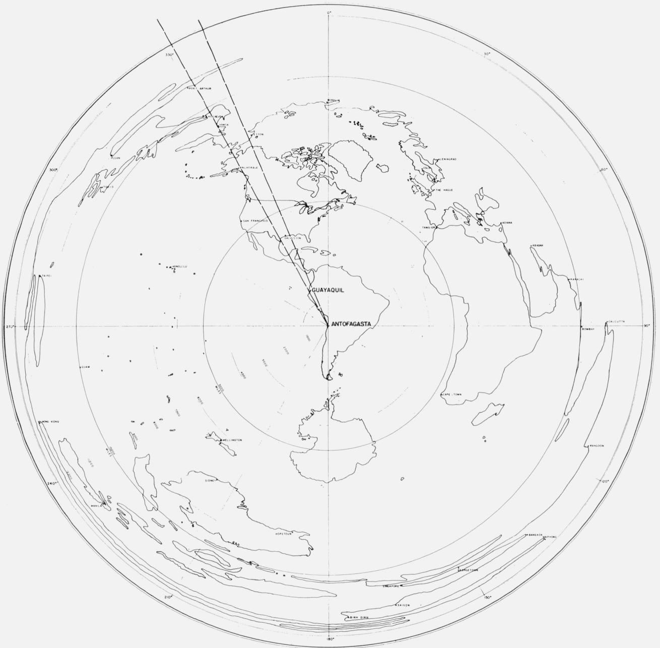
FIGURE 3. Polar plot of the world centered about Antofagasta, Chile, showing coverage of the principal antenna beam.
