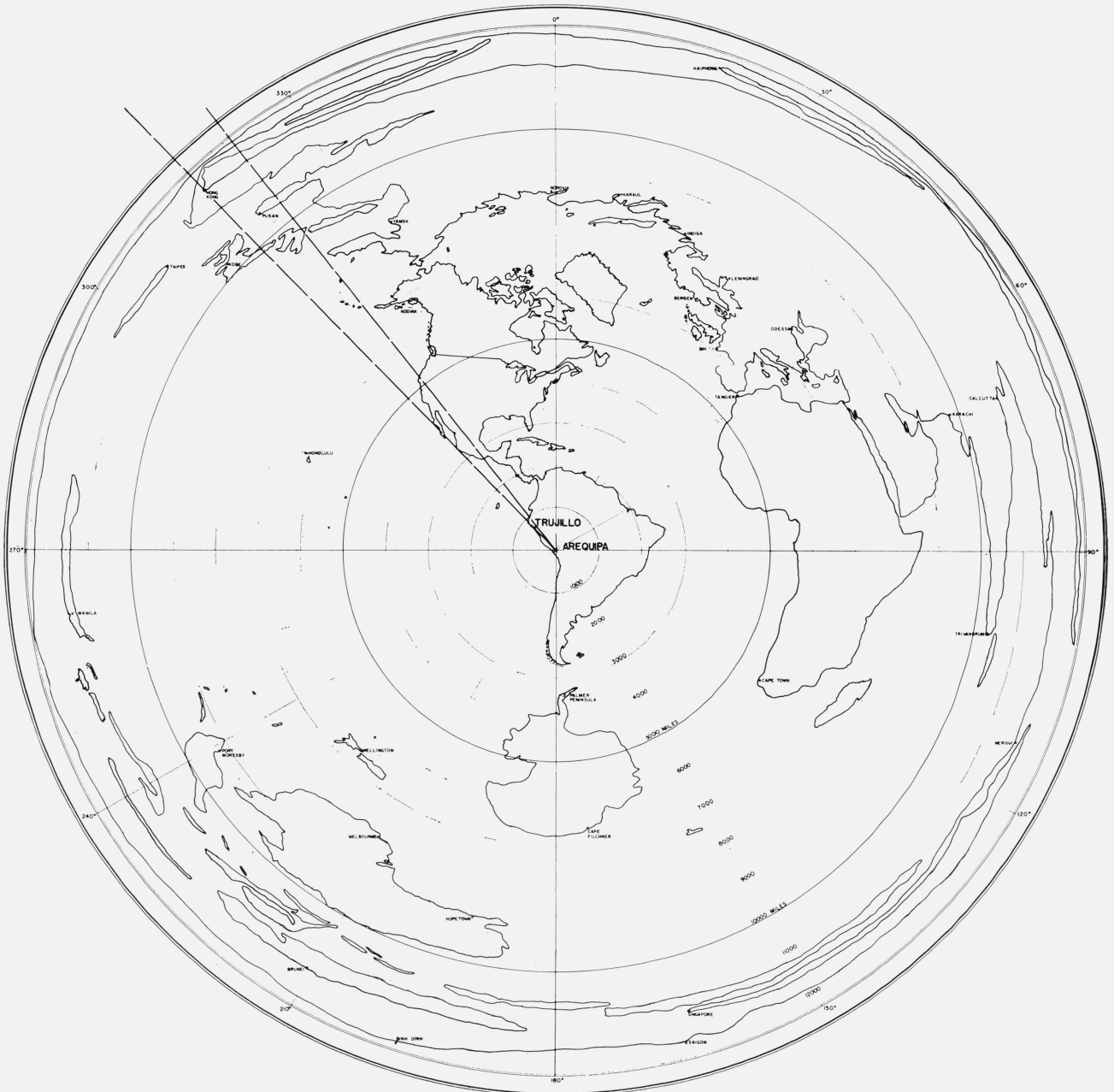
FIGURE 4. Polar plot of the world centered about Arequipa, Peru, showing coverage of the principal antenna beam.
