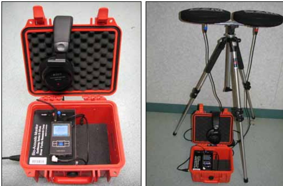
Figure 9: Field configuration of the E3A Bioacoustic Monitor recording unit using a stereo configuration with two 180° CZM microphones.
