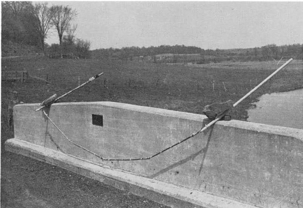
View of alternate-polarity electrode in extended position.
