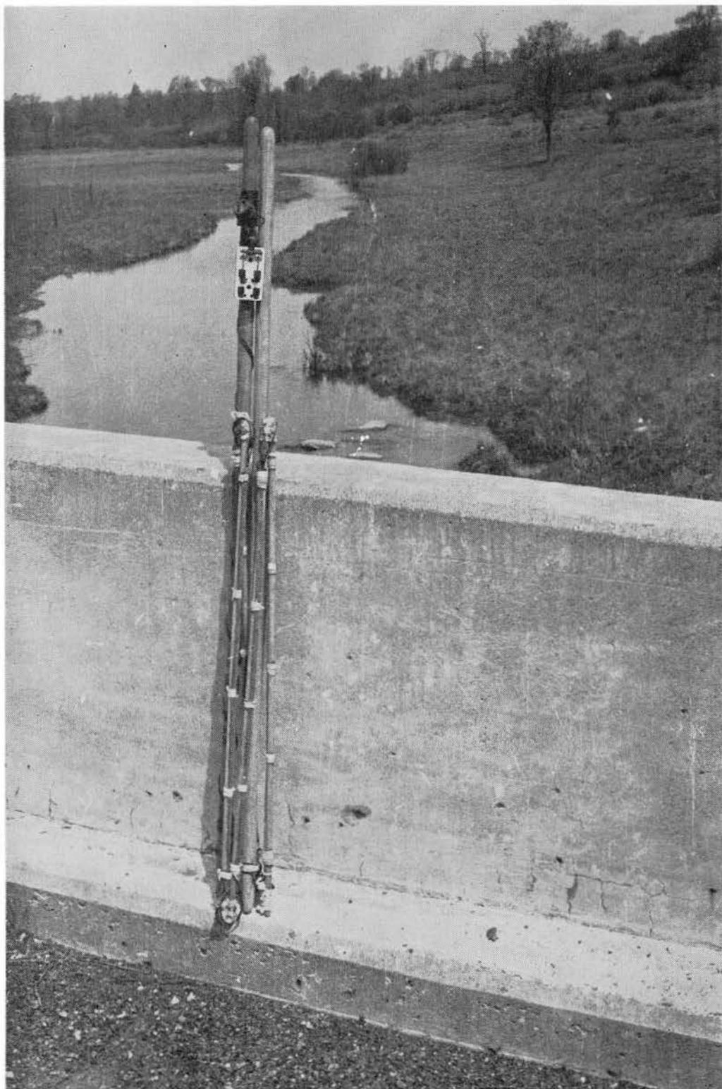
View of alternate-polarity electrode in folded position showing switch and connection for power source.
