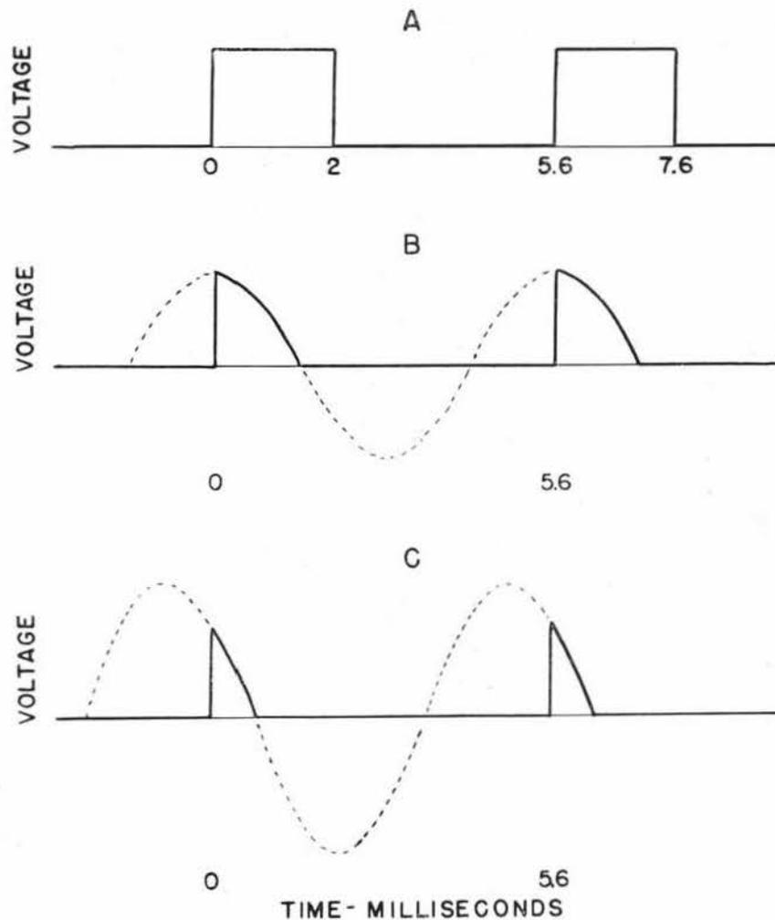
Figure 5. Types of wave or pulse studied in connection with rapid and combined cycles: A, square wave; B, quarter-cycle sine wave; C, eighth-cycle sine wave.
