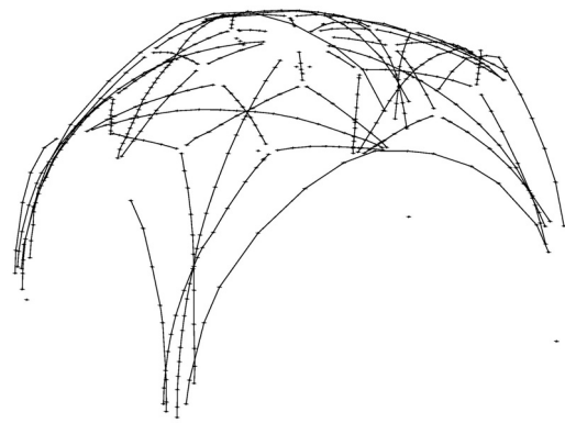
Fig. 6: Result of the topographical measurement of the vault.
