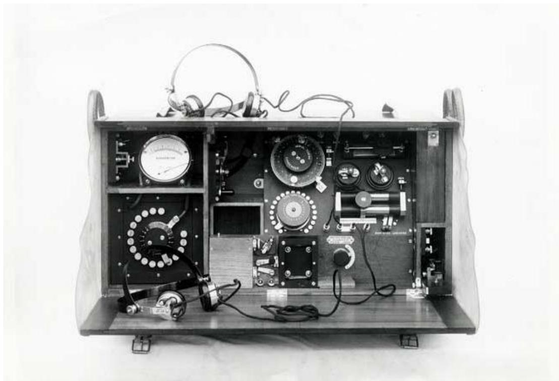
Figura 7.8 ¼ kW Marconi Wireless Pack Set, modelo B1. 1918
