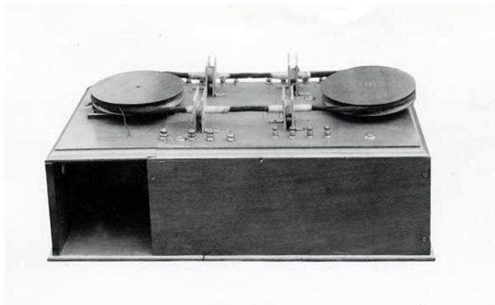
Figura 4.15 Detector magnético, 1902. Fuente: <http://www.marconicalling.com/introstring.htm>
