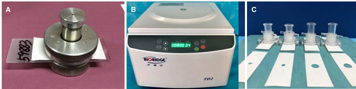
Figure 1. (A) The Hou's chamber modified from the Sayk's method which is still in use in some CSF labs in China; (B) the cytocentrifuge equipment for the Su's Centrifugal method (photo provided by Yi-Ning Yang from Xijing Hospital); (C) the chambers used in the Su's Centrifugal method (photo provided by Yi-Ning Yang)
