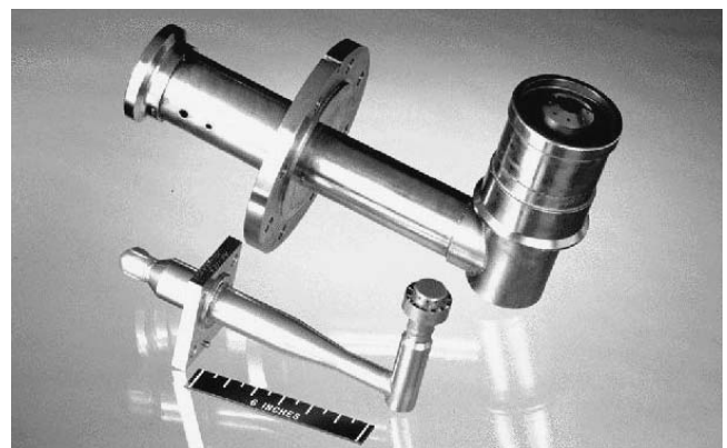
Figure 11. Conventional and Lean Premixed Fuel Injectors.
