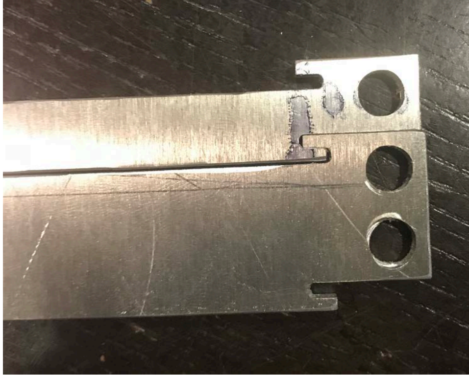
Figure 8. Interlocking method on aluminum fabrication.
