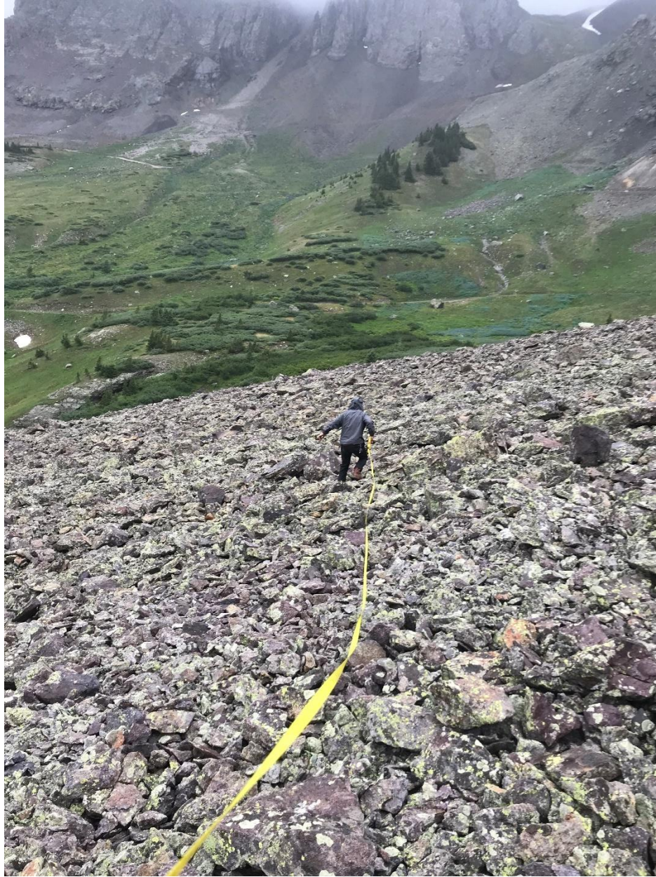
Fig. 9 - Field work conducted at the Camp Bird rock glacier July 2020. Transverse profile measurements were manually collected with GPS data and a 100 ft tape measure. Photograph captured by field assistant Jacqueline Rambo, July 2020.
