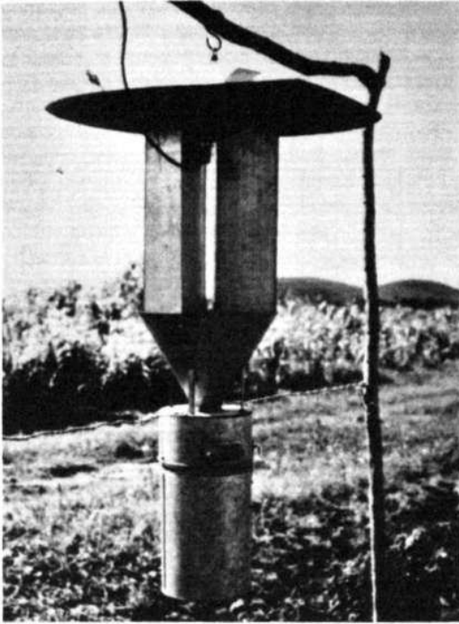
Figure 1c. Light trap for collecting H. zea adults for laboratory colony establishment or renovation.
