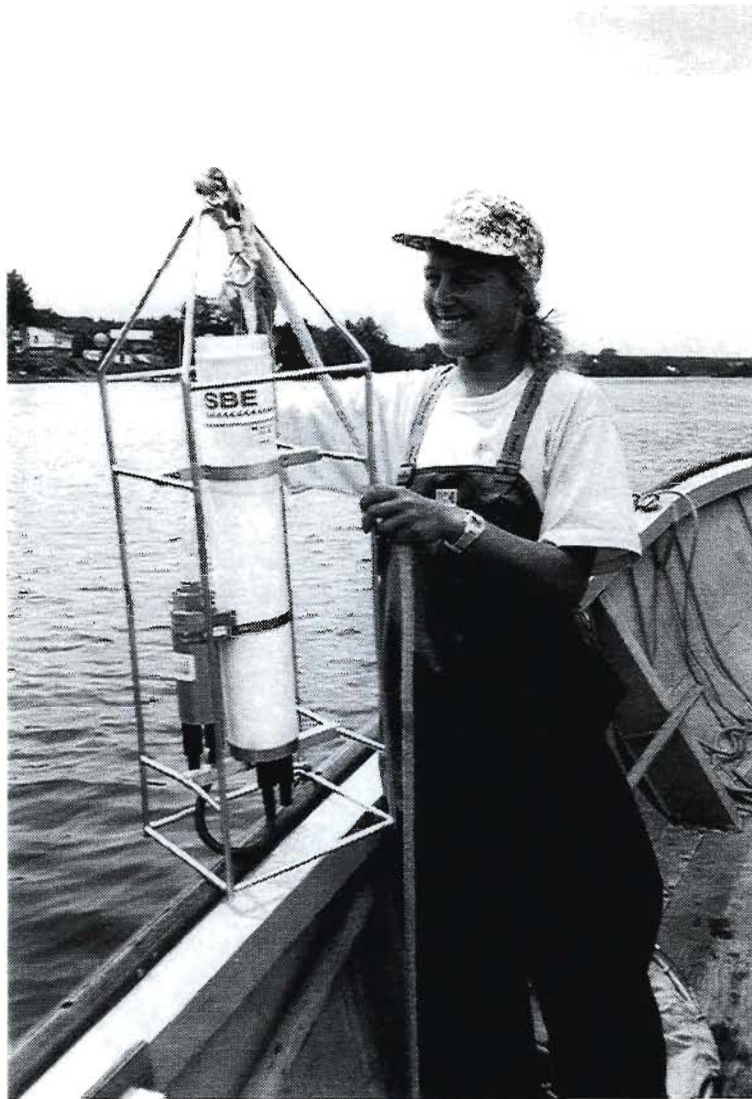
This instrument is used to measure conductivity (salinity) and temperature at various depths of the water column. Salinity profiles are used to describe the location of features like the salt wedge in Miramichi Estuary.
