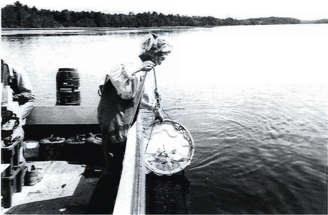
A plankton net is used to collect small organisms in the upper parts of the water column. This type of equipment was used to collect larval fish and zooplankton throughout the Miramichi Estuary.
