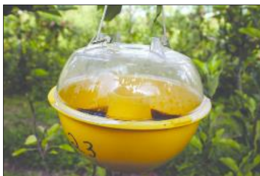
Figure 6 McPhail model trap recommended for monitoring Anastrepha fraterculus (Wiedemann, 1830) (Diptera, Tephritidae) and Ceratitis capitata (Wiedemann, 1824) (Diptera, Tephritidae); (Source: https://www.researchgate.net/figure/Figura-4-Armadilha-modelo-McPhail-recomendada-para-o-monitoramento-de-Anastrepha_fig2_305073720 )
