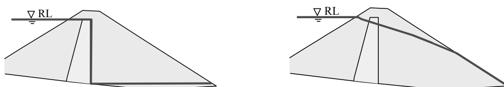
Figure 3: Normal ground water pressure (left) and assumed water pressure at design leakage (right)
