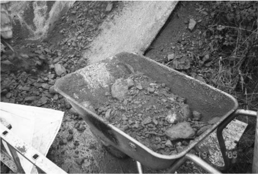
Figure 5: Sampling glacial till used for shoulder fill
