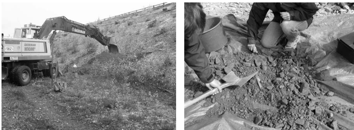
Figure 4: Test pit at the down stream toe at a typical rock fill dam. Determination of content of material 0-60, 60-120, 120-200 and > 200 mm in the field.
