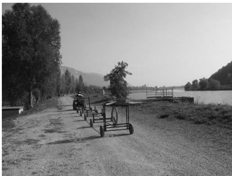
Figure 1: Fast EM® investigation device with mounted EM34
