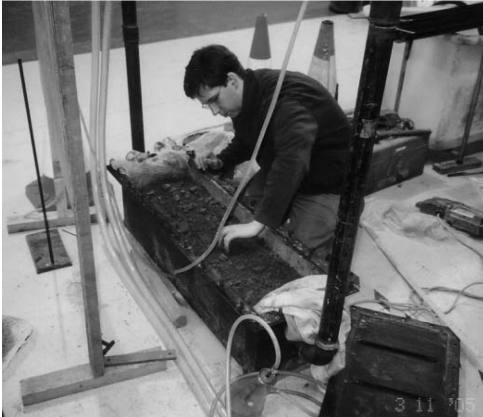
Figure 4: TRL (formerly Transport and Road Research Laboratory) 0.3 m square by 1.0 m long permeameter.
