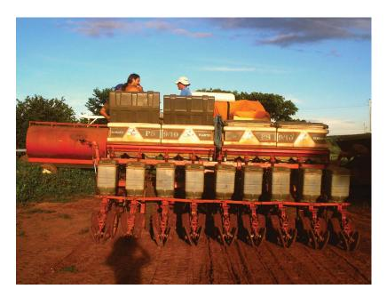
**FIGURE 6** Planter machine used for direct-seeding in-rows, Mato Grosso State, west-central Brazil (Credit: Luciano Langmantel Eichholz) (color figure available online).
