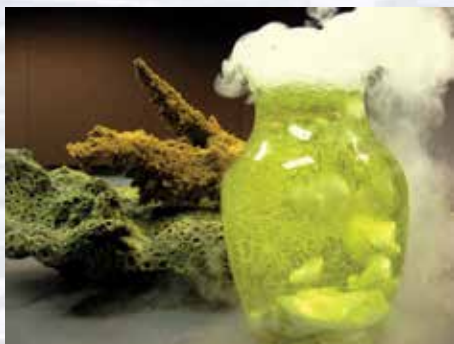
Dry ice, a pH indicator, and water can be used in the classroom to demonstrate the acidifying effects of carbon dioxide in ocean water. For a similar demonstration using human respiration instead of dry ice, see page 41. Image credit: NOAA/CRCP
