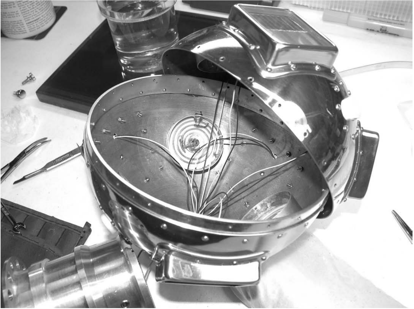
FIGURE 11. Inspection of a replica of Vanguard 1 that had been modified to hold a solar powered audio system for demonstrating the “beeping.” (NASM photograph)
