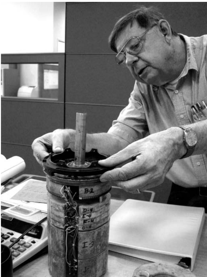
FIGURE 5. George Ludwig examining his engineering model for the payload for the first fully instrumented Vanguard flight and became the template for the Explorer 1 payload. (NASM photograph by Dave DeVorkin)
