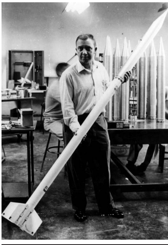
FIGURE 10. James Van Allen holding a balloon-launched Loki-Dart payload developed at Iowa. (James A. Van Allen Papers, The University of Iowa Libraries, Iowa City, Iowa; c. 1950s)
