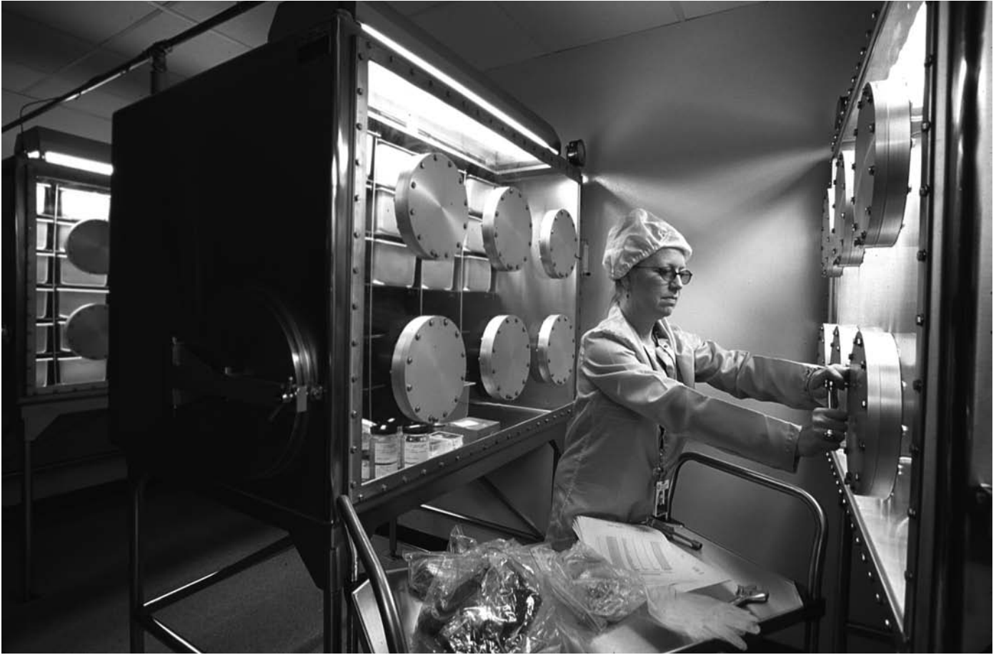
FIGURE 4. Meteorite storage laboratories at the Smithsonian Museum Support Center in Suitland, Maryland, modeled on the facility used for lunar rocks at NASA's Johnson Space Center. The water- and oxygen-free nitrogen gas in the cabinets keeps meteorites from oxidizing and free from contamination by environmental pollutants such as organic compounds, heavy metals, and salts, which could reduce the scientific value of the specimens. Photo by Chip Clarke, SI.
