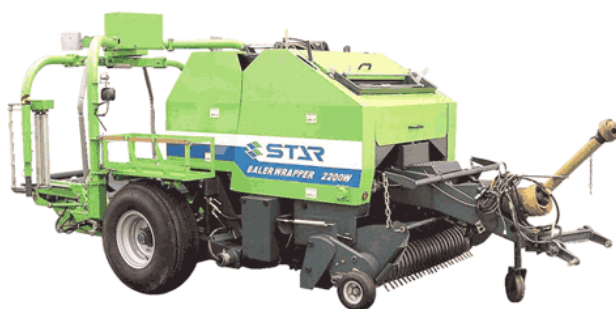
Fig. 6-29. Roll Baler with Rapping Machine System.
