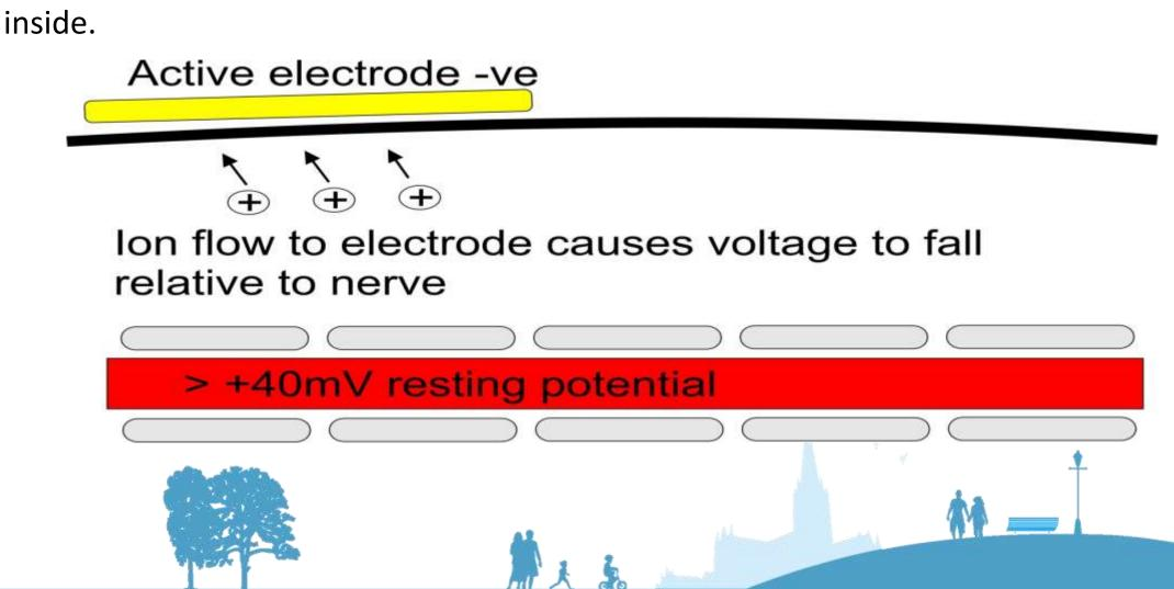
Once the voltage falls enough so the inside of the nerve becomes 40mV positive relative to the out side and the threshold is passed to open the ion channels. This causes an action potential.
