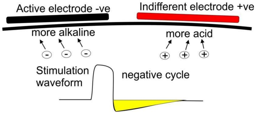
Over the whole stimulation cycle the ion flow is balanced and hence the balance of acidity and alkalinity is also balanced. However, threshold effects may prevent perfect balanced charge.
