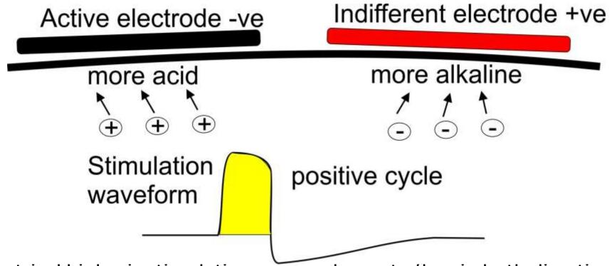
Asymmetrical biphasic stimulation causes charge to flow in both directions.
