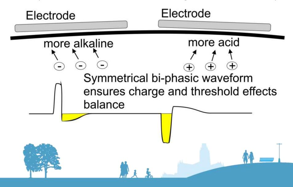
Symmetrical biphasic waveform may be less irritating to the skin Electrode Electrode more acid more alkaline symmetrical bi-phasic waveform ensures charge and threshold effects balance
