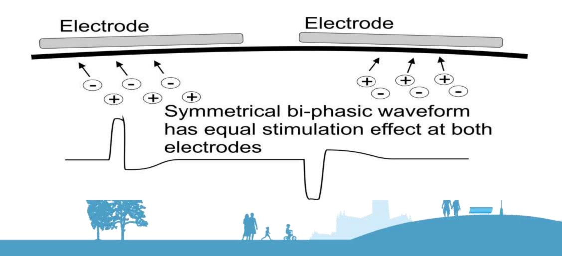
**Standard electrode position with SYMM waveform.** Electrode 1 stimulates dorsiflexion and Eversion. Electrode 2 stimulated dorsiflexion and inversion.
