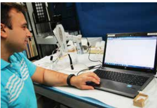
Figure 3. Shaheen Chaudhri uses the Bruker Tracer XRF spectrometer to analyze clay tablets from Persepolis
