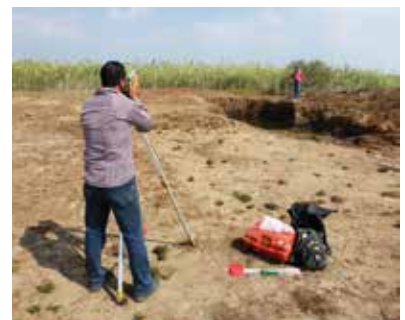
Figure 12. Inspectors Ahmed and Ibrahim learning the use of the Leica Total Station for setting a grid on Zone 6 (photo: G. Marouard)
