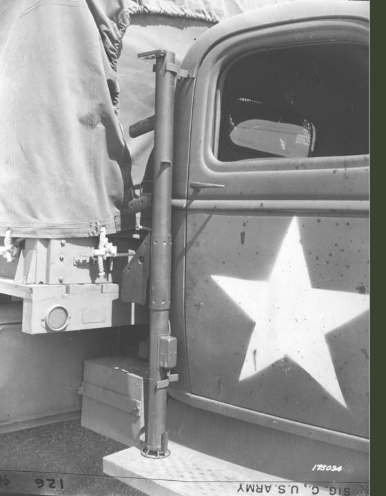
Rocket gun mounted on a 1/2 ton vehicle. Camp Gruber, Okla. 4/3/43; 788th Ordnance (111-SC-175034)
