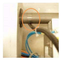
Hydraulic Line Wearing in Contact With Rotating Shaft
