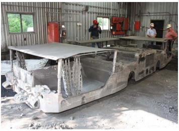
Above, the mantrip in which the Tailgate 22 crew was riding; below, the remains of a cinderblock wall gives an indication of the force of the explosion.
