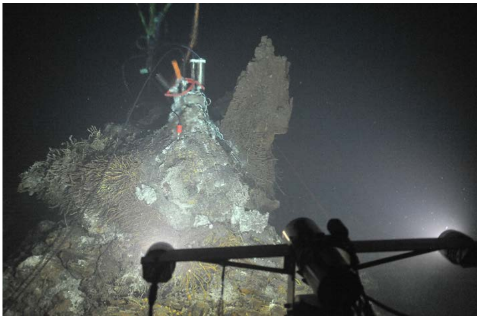
FIGURE 10.1 The RCA cabled digital still camera, redeployed in 2015 by the Canadian ROV ROPOS, lights up the active hydrothermal vent called El Gordo in the interantion District Hydrothermal Field, located at the summit of Axial Seamount nearly a mile beneath the ocean surface. Credit: UW/NSF-OOI/CSSF.
