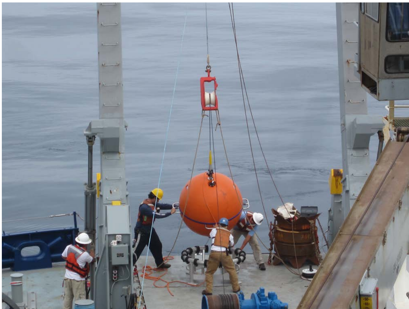
FIGURE 2.3 Deployment of the main float of the Profiler Mooring from R/V Melville at the Global Station Papa Array. Credit: Station Papa Science Team.
