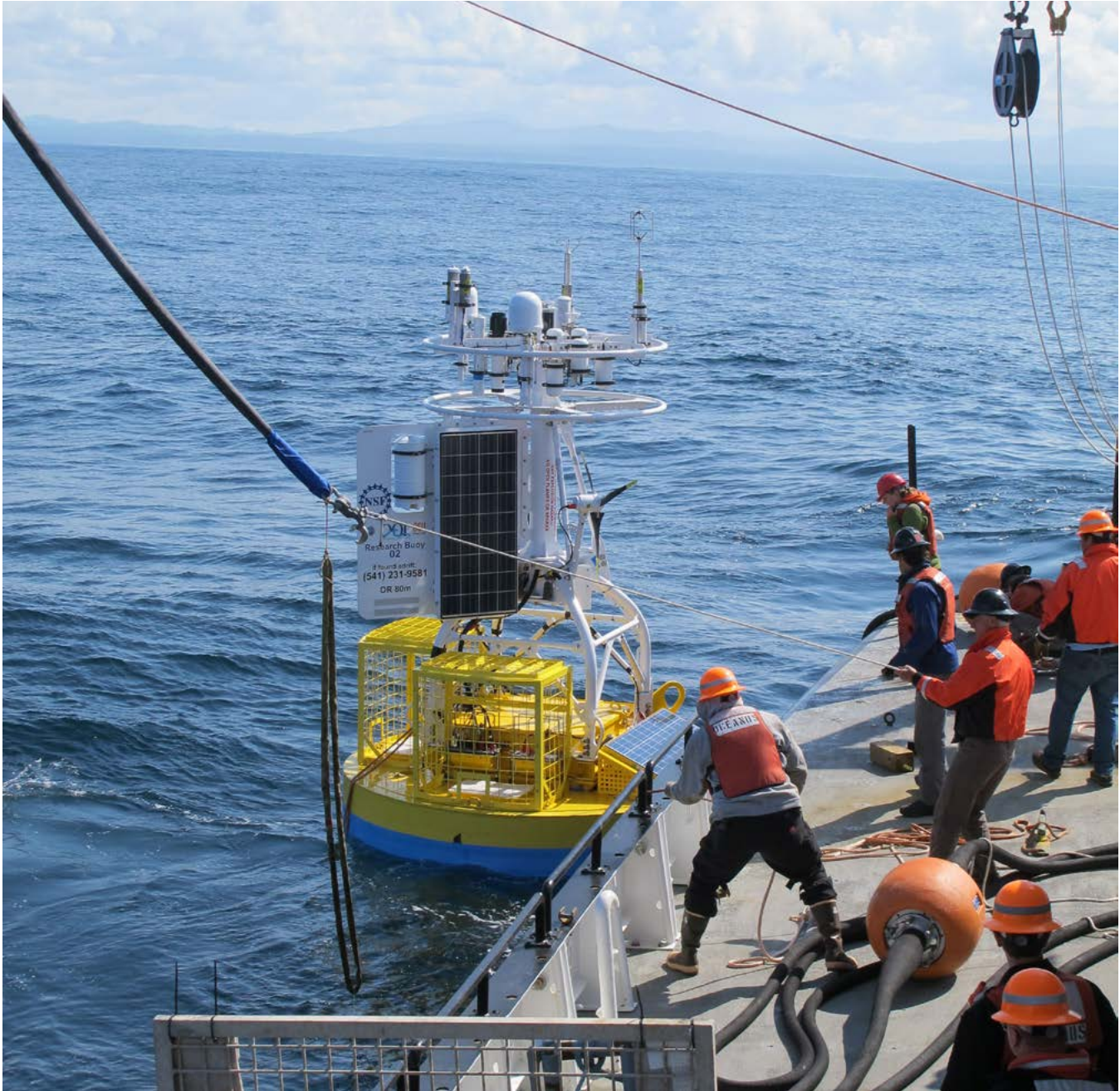
FIGURE 4.2 The Oregon shelf surface mooring is released from the crane by EA science party field chief, Walt Waldorf. Credit: OOI Endurance Array Program, Oregon State University.
