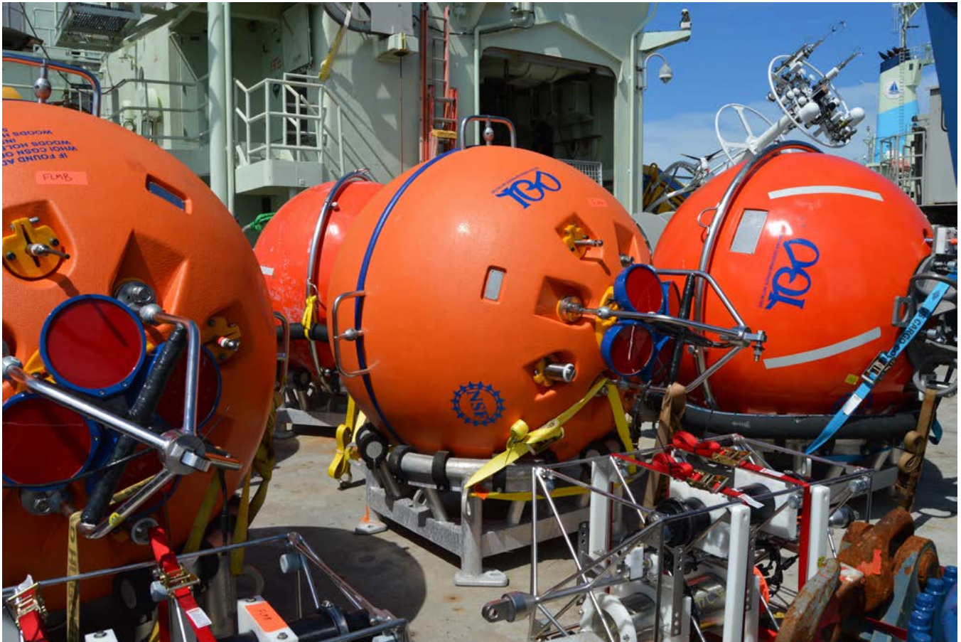
FIGURE 1.3. Sub-surface floating spheres and controllers for two flanking moorings and the Global Profiling Mooring await deployment in the Irminger Sea Array. These instruments measure water velocity from the depth of the spheres (500 meters) to the sea surface. Credit: Sheri N. White, Woods Hole Oceanographic Institution.
