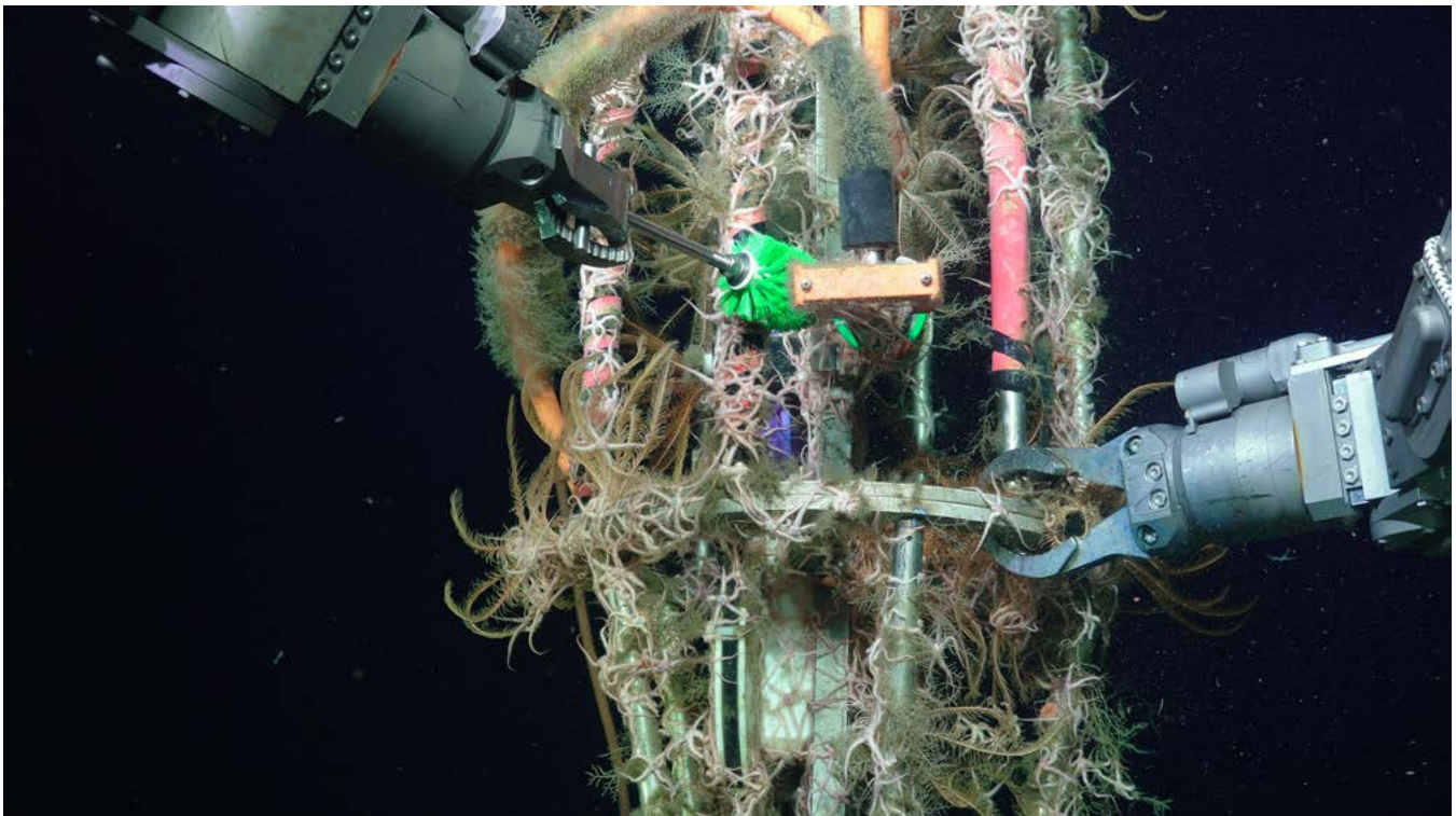
FIGURE 2.9 Brittle stars and feather stars encase a wet-mate connector frame on the Oregon Offshore Shallow Profiling Mooring Leg in ~ 210 m water depth. Credit: University of Washington/National Science Foundation-OOI/Woods Hole Oceanographic Institution: V19.
