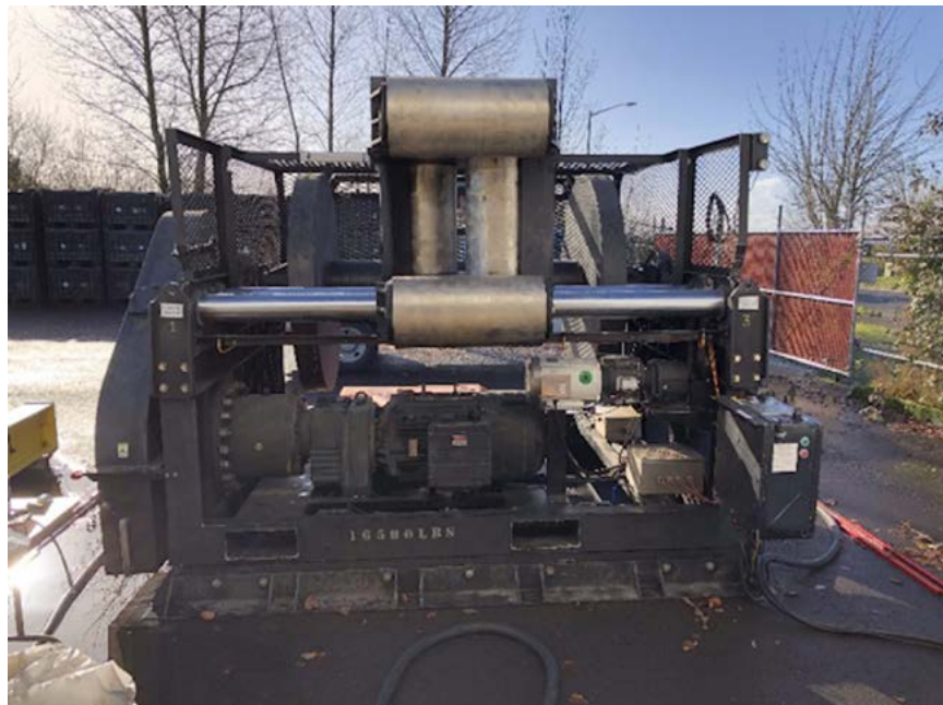
FIGURE 5.7 Heavy Lift Winch. Credit: Jonathan Fram, Oregon State University.
