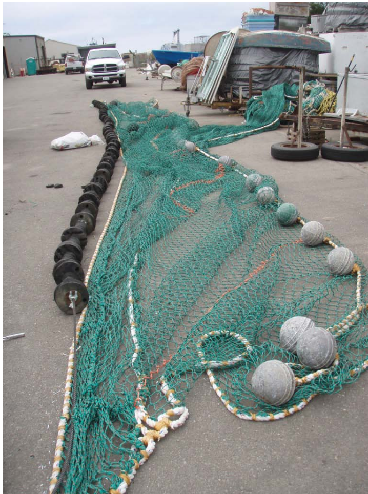
Figure 2. Picture showing the footrope and groundgear (left) and the headrope with attached floats (right).
