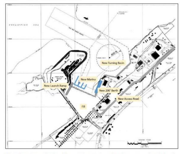
This configuration was abandoned due to environmental permitting issues, cost, and terminal needs. Subsequent coastal engineering analysis of wave and current monitoring data showed that an enlarged turning basin would not improve vessel navigation. Cargo forecasts also showed that additional backland terminal area would not be needed to support the commercial port operation at Rota West Harbor.
