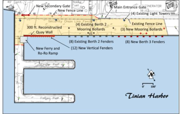
With the Ro-Ro ramp available at Berth 1, the remainder of the Connecting Pier along with both Finger Piers would be closed to further use. In addition, the upland area is cleared of non-essential fencing and damaged portions of the Berth 1 pavement will be razed and repaved. Soil and vegetation is cleared from operations areas along the wharf, and high-mast lighting is repaired to allow night operations.
