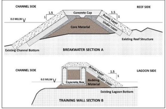
Figure 6-5: Typical Breakwater and Training Wall Section
