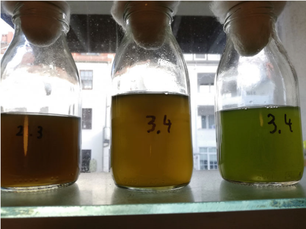
Fig. 5 Simple algae culturing unit using natural light without shaker. Bottles are shaken manually once every working day because algae tend to settle on the bottom. Isochrysis sp. (left bottle) and Nannochloropsis sp. (right bottle)
