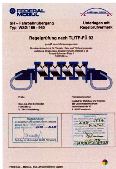
Figure 4.1 'Regelprüfung'-document for WSG-type girder grid joints.
