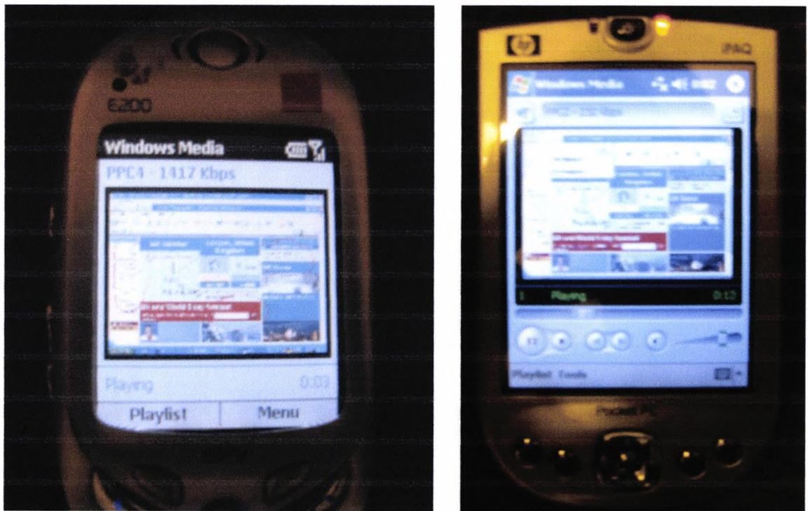
Figure B.7 and B.8. VIVID screenshot replaying a VIVID encoded clip, with audio encoding, tested on an SPV E200 Mobile phone and an HP Ipaq 4150 PocketPC
