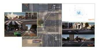
Figure 1: Illustration of multi-agent hetero-modal V2V systems where each agent may be equipped with either LiDAR or multi-view cameras.
