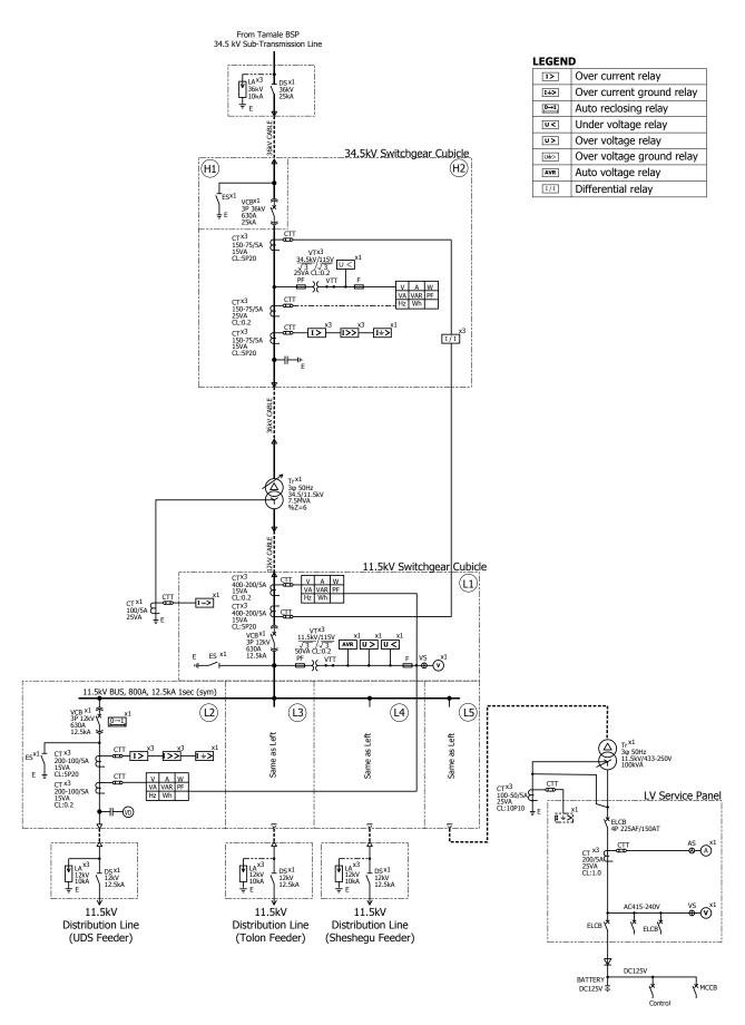
Fig. 2-2-3.2 Single Line Diagram of UDS Primary Substation
