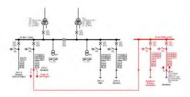
Fig. 2-2-3.12 Single Line Diagram of Sunyani BSP Substation
