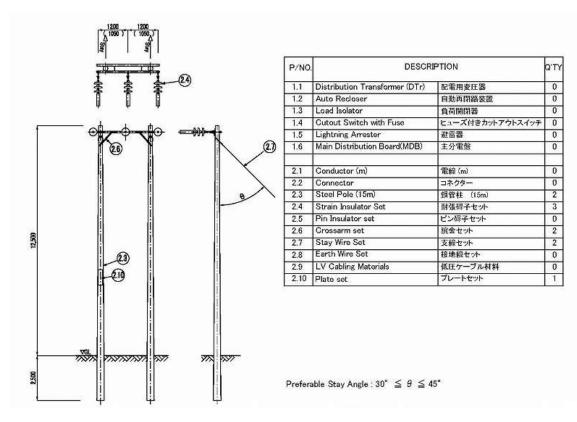
Fig. 2-2-3.27 34.5/11.5 kV Terminal Pole
