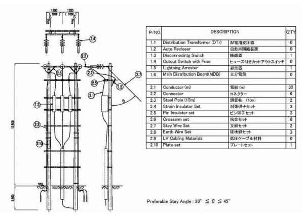
Fig. 2-2-3.29 34.5/11.5 kV Disconnecting Switch Pole (Vertical Dead End Type)
