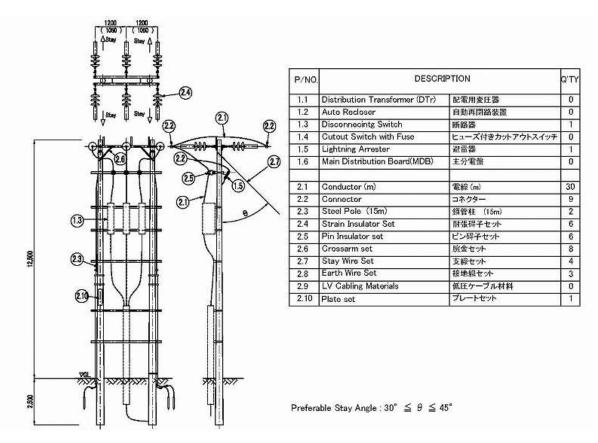
Fig. 2-2-3.30 34.5/11.5 kV Disconnecting Switch Pole (Vertical Section Type)
