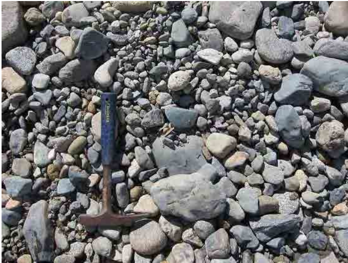
Photo-3 Gavels which cover the riverbed is suitable for concrete aggregate.
