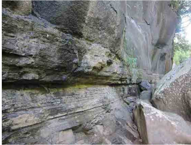
(Photo-4) Geological condition surrounding the dam site is Rock characteristics of massive sandstone and grooved mudstone. Even though some layer of
