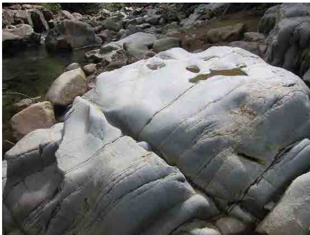
Photo 0-8 Fresh and hard Andesite on the right bank riverbed of the proposed dam site
