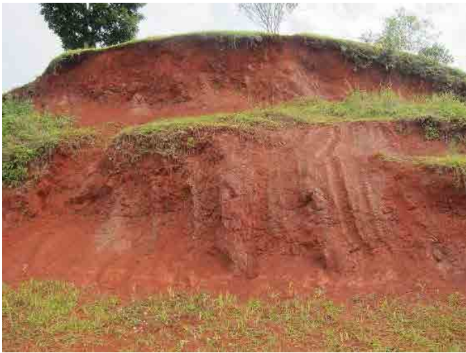
Photo-1 - Weathered outcrop is observed in a cutting slope behind the playground of Dawara village elementary school Strike and dip of the strata is N25W/70NE.
