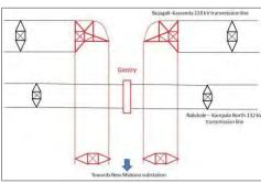
Figure 2-3: Image of overpassing method
