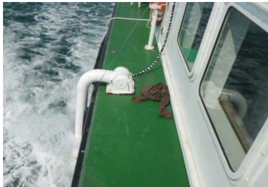
Transducer of MBES mounted with gunwale
