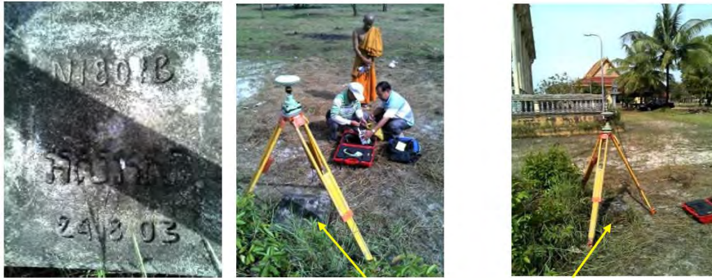
Photo 2 - 1 GNSS Observation at National GPS Point 1801B
