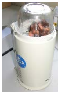
Fig.2 Chopping of the sample using grinder
