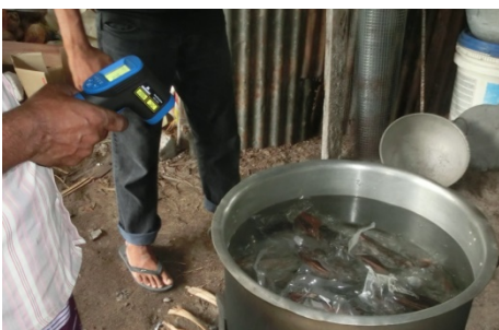
Fig.4 Measuring water temperature using infrared thermometer
