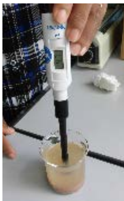
Fig.12 Measurement of pH using pH meter
