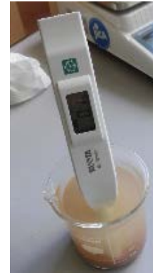
Fig.11 Measuring salt content using electronic salt meter
