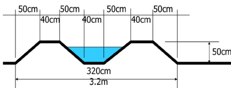
**Figure 4.1.3 Typical Cross Section of Main Farm Ditch (Left) and Typical Supplementary Farm Ditch (Right)**
