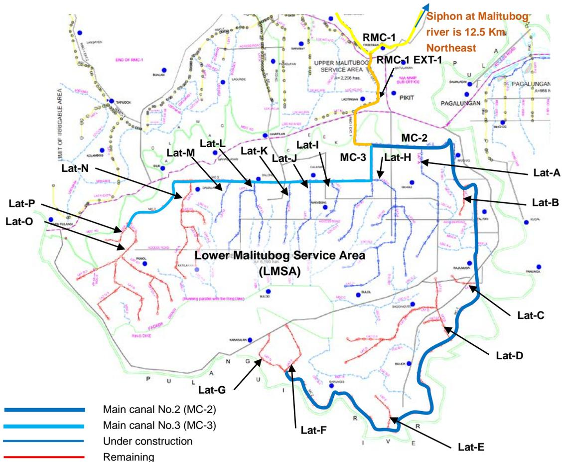
**Figure 4.3.9 Plan of Irrigation Canal System for LMSA**
