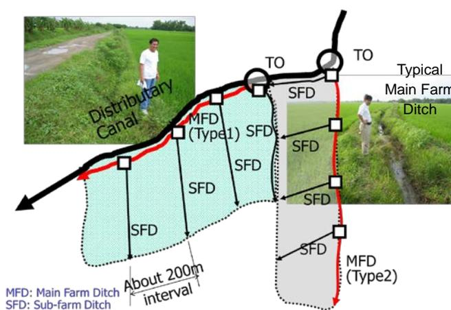
**Figure 4.1.2 Typical On-farm Ditch Arrangement**
