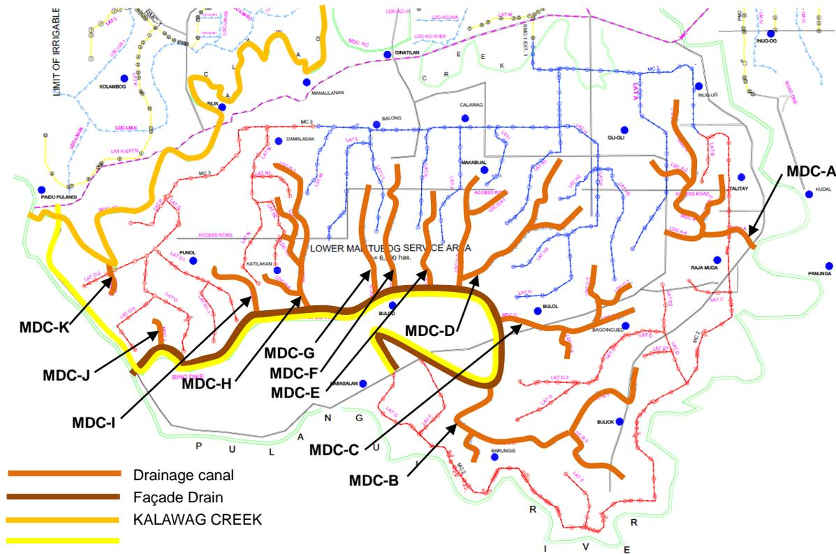
**Figure 4.3.11 Plan of Drainage Canal System for LMSA**
