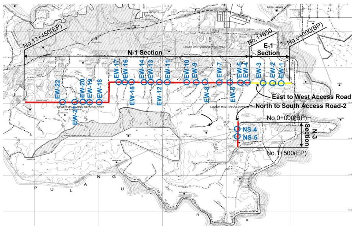
**Figure 4.4.6 Location Map of Access roads and Bridges (Construction Plan of Case-1)**
