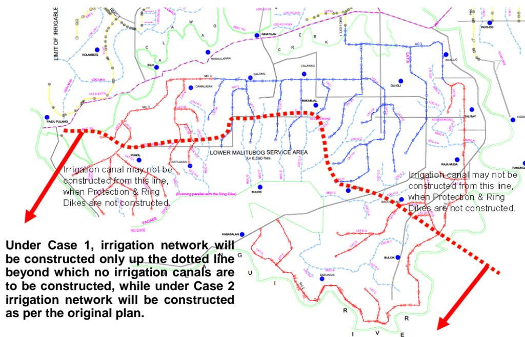
**Figure 4.1.4 Conceptual Irrigation Development of Case 1 and Case 2**
