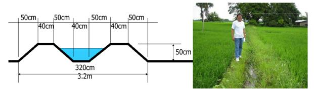
Figure 4.1.3 Typical Cross Section of Main Farm Ditch (Left) and Typical Supplementary Farm Ditch (Right) Source: JICA Survey Team
