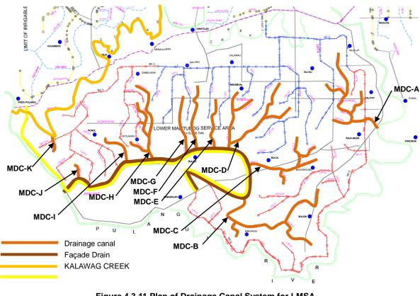
Figure 4.3.11 Plan of Drainage Canal System for LMSA Source: NIA-PMO, JICA Survey Team
