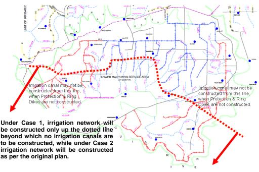
Figure 4.1.4 Conceptual Irrigation Development of Case 1 and Case 2 Source: JICA Survey Team
