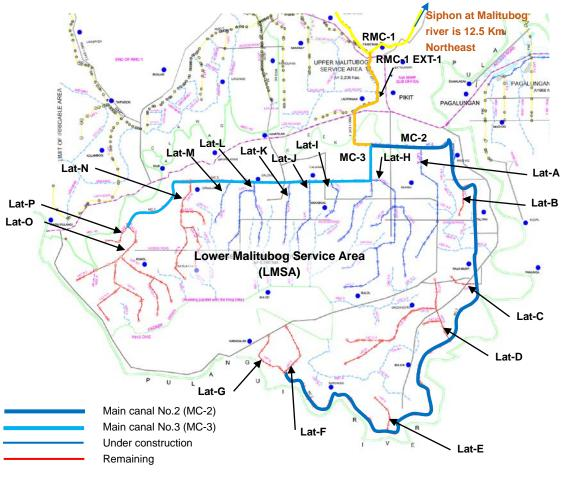
Figure 4.3.9 Plan of Irrigation Canal System for LMSA Source: NIA-PMO
