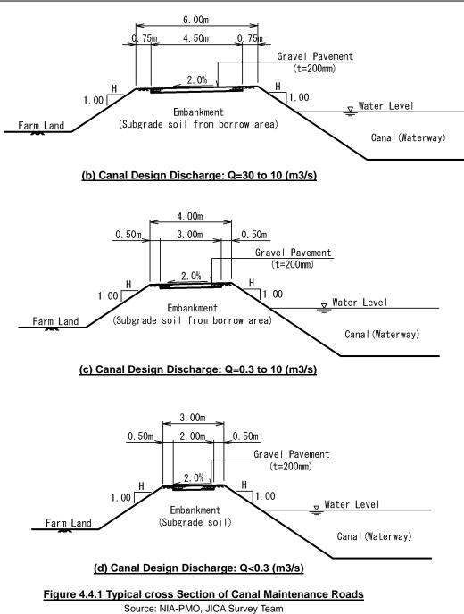
Generally, roadway cross slope is slightly to be slanted from the road center to the both sides (convexity shape) in order to drain the road-surface water (rainwater etc.). However, the crossing gradient of canal maintenance road keeps 2.0%, down from the canal side (water side) to farm land side in order to prevent the road-surface water from flowing into the waterway/ canal section. Figure 4.4.1 shows the typical cross sections of canal maintenance roads by NIA's own design standard.
