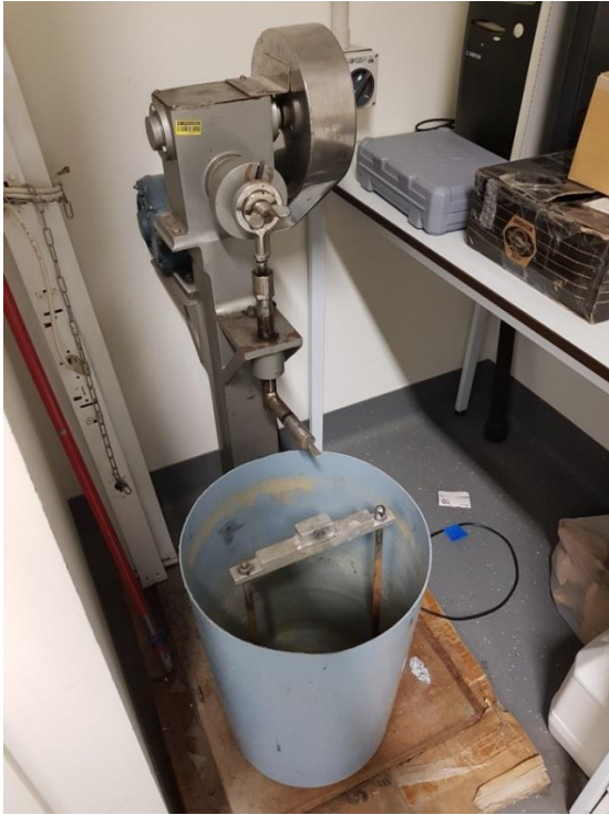
Figure 10. Machinery used to process sediment sample in the centre of the image. Seven sieves were held and rotated through water.
