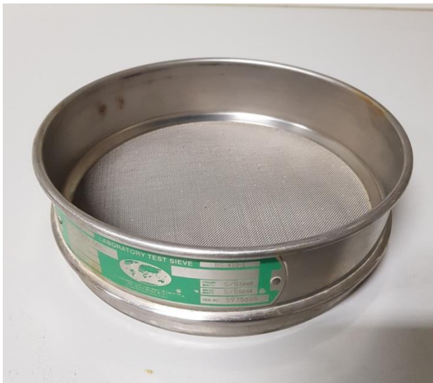
Figure 11. Example of one of the seven sieves used to separate sediment samples. (500 microns.)
