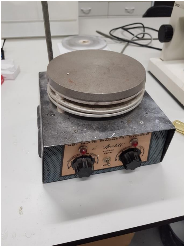
Figure 4. The hot plate used to melt the CrystalBond adhesive and thus mount the sample section to the slide.
