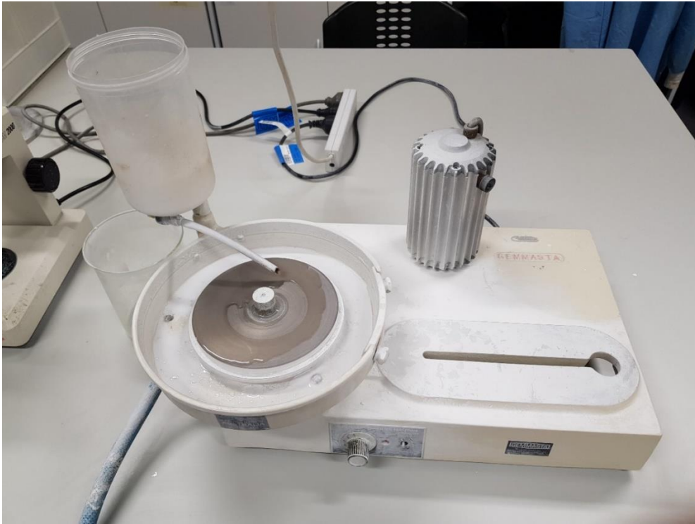
Figure 6. The Gemmasta polishing wheel used to polish the samples to the desired thickness with the water input device visible.
