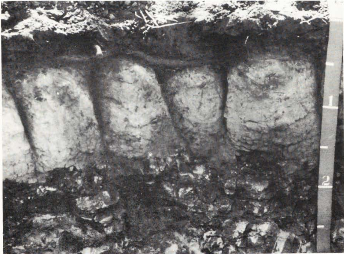
Plate 7 Solodised solonetz showing the distinctive coarse columnar structure and bleached A_2 horizon penetrating between the columns. The strong and abrupt texture change from A to B horizons is common to a wide range of texture-contrast soils (CSIRO photo)
