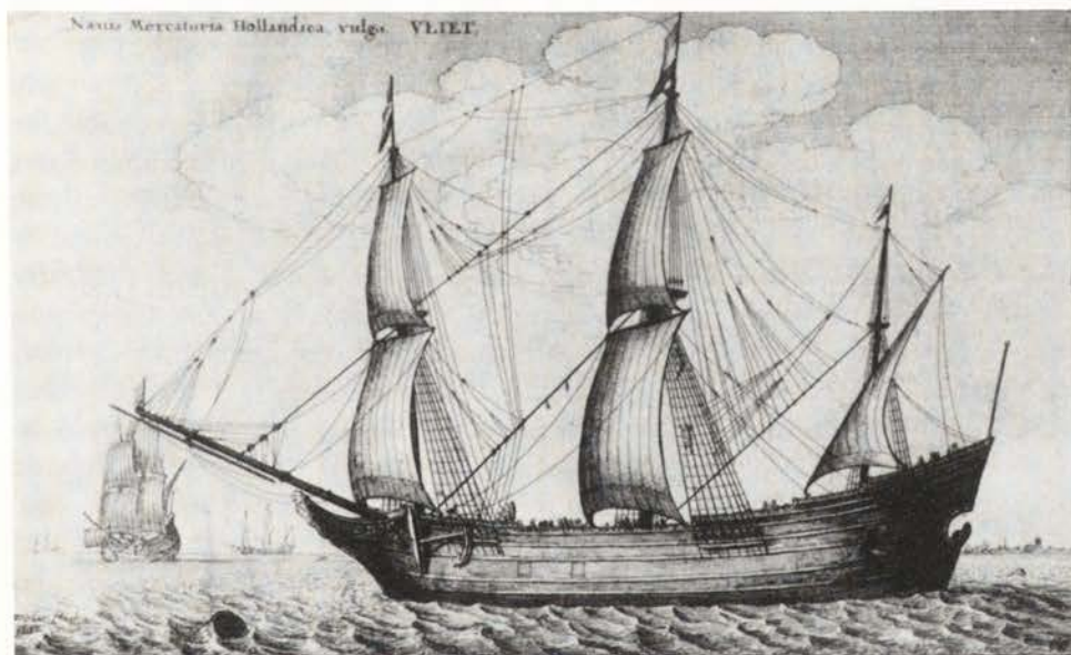
Plate IV. DUTCH FLUYTS. Roomy and cheap to build and work, the fluyt (English 'flyboat', French 'flûte', Spanish 'felibote') was much used as a general service cargo vessel from the later sixteenth century onwards. From R. Davis, English Merchant Shipping and Anglo-Dutch Rivalry in the Seventeenth Century (London 1975), by permission of the National Maritime Museum, London. ANU.
